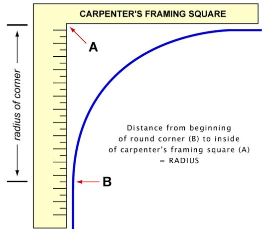
Above is an illustration of the best way to measure the radius. With a carpenter's framing square, you need to "square" out the corner. What will result is the framing square representing where the corner would be if the corners were not rounded.
